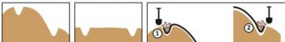
EN - Dig a trench on top and at the base of the slope. Dig a trench on the sides. Start filling the trench on top. Pull straight & fill the trench at the base.
