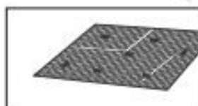
EN - Use 2x30cm anchors/m<sup>2</sup> on slopes >2:1. Use 1x20cm anchors/m<sup>2</sup> on flat surfaces. Or use pins.
