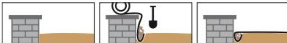
EN - Ökolys next to a wall, fence, ... Make a groove right next to the obstacle for groundcover. Pull the groundcover straight.
